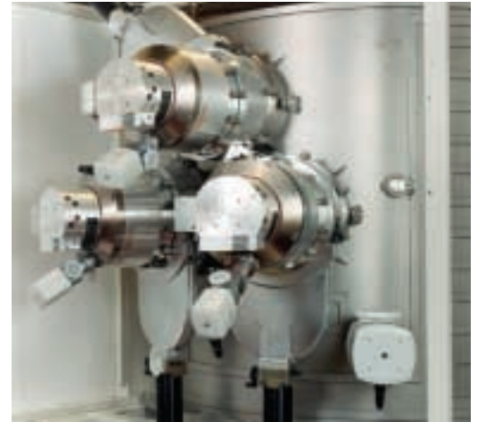
Ophthalmic Coaters Deposition of anti-reflection films on lenses. Photo: Courtesy of Satis, Italy
